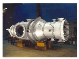
A.H. Lundberg supplies surface condensers for many different types of gases and operating conditions. Horizontal and vertical orientation designs are given consideration. Condensers may be designed on a "stand alone" basis or be interated into a mass transfer column.
