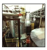
Where low pressure steam is not available, A.H. Lundberg Systems offers single effect falling film concentrators with mechanical vapour re-compression to power the evaporation process. Although "starting steam" is required to start the evaporation process, re-compression and re-use of the steam/vapour produced from the liquor itself, is used as the heat source to maintain the evaporation process.
