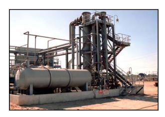
The decanter and storage tank is used where it is necessary to remove an immiscible lower density fluid from another higher density fluid. The decanter is sized to provide sufficient residence time for the immiscible fluid to separate, then be skimmed off and stored.
