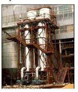
A.H. Lundberg Systems' preferred technology for crystallizing solids from liquor or brines is "Flooded Forced Circulation". This technology utilizes forced liquor circulation through the tube side of a heater with the liquor under a back pressure to suppress boiling. The superheated liquor is flashed in a vapour head, resulting in evaporative cooling.
